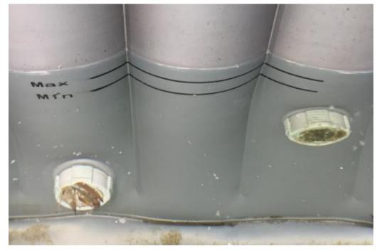
Reason 2: The hose connecting the inside and outside of the Liner is not straightened, or the hose is flattened, which reduces the water flow speed.
