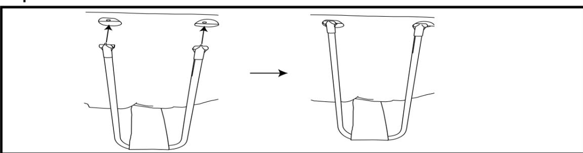
Find the one side holes on the horizontal beam.Place and lock the T-joints into the holes.Ensure they are fully connected
